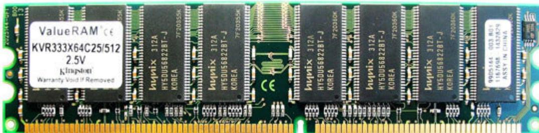
Figure . A 512 MB DDR RAM module.
